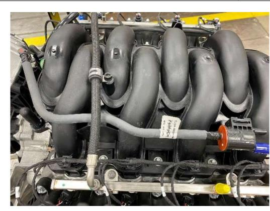
Run and secure the wire for the crank shaft speed sensor as shown:
