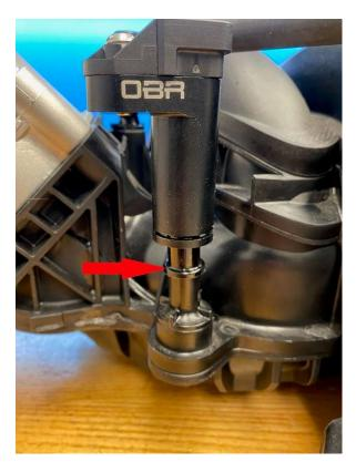
Carefully push the adaptor down onto the nipple, make sure the adapter slides all the way down over the nipple. The collar marked with the red arrow must be inside the adapter and above the slot.
