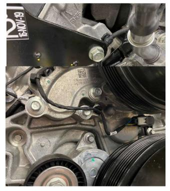
Run and secure the wire to the oil pump control as shown:
