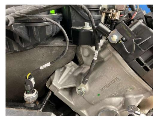
**Warning:** Make sure you have connected your battery's negative terminal to chassis ground AND that your engine also has a wired connection to the car chassis.
