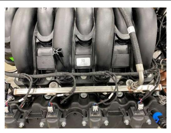
Secure the leg with the oil pump control, CHT, VCT, ETB and the cam sensor connectors to the intake manifold and run the 'ETB' cable to the throttle body:
