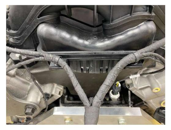
Start on bank 1 and lay the harness along the fuel rail, on the side towards the intake manifold. Run each pair of coil and injector connectors over the fuel rail and plug the connectors into the injectors and coils. Push the lock on each connector forward to secure its location. Cylinder '1' is at the front of the engine.
