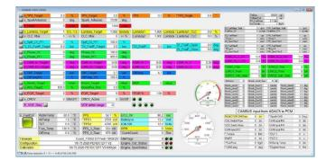
In this example you see that the programmed oil pressure target is 0.7 bar. A different pressure target has been entered in the window on the right, named '**v\_OilP\_Target**'. By pressing the button marked in yellow this new target for the oil pressure has been applied and the data window for oil pressure shows the new value.
