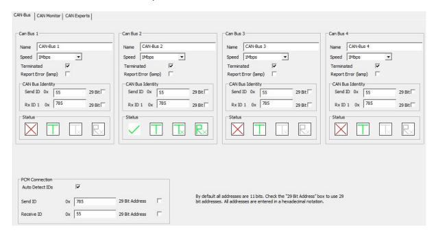
The CAN display screen shows status for each of the 2 CAN bus:
