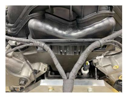
Start on bank 1 and lay the harness along the fuel rail, on the side towards the intake manifold. Run each pair of coil and injector connectors over the fuel rail and plug the connectors into the injectors and coils. Push the lock on each connector forward to secure its location. Cylinder '1' is at the front of the engine.
