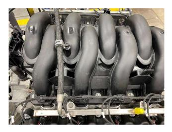
Carefully push back the white lock in the hose connector, the hose can now be removed from the nipple on the intake manifold. Slide the Bosch TMAP adapter and sensor onto this nipple, push it all the way down and fit the lock spring to lock it in place. Plug the 4-way connector with the orange seal into the sensor.
