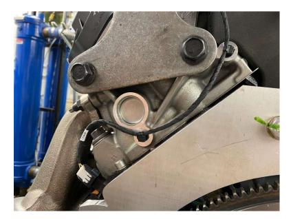
Connect the wire to the oil pressure sensor and fix the ground terminal to the cylinder head with the supplied fastener.
