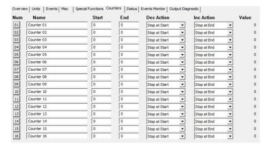
This section is used to define PCM2's ability to count sequences.
