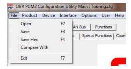
You can display differences between two configuration files by selecting the function COMPARE WITH. Please refer to section 6.
