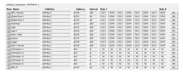
The opening screen displays the general setting for 16 CAN export channels on each of four pages.
