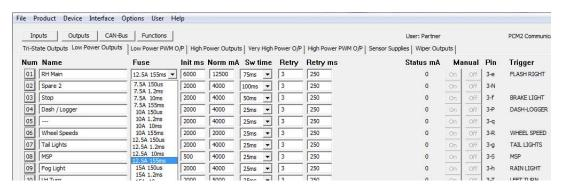
Current draws can be measured on all outputs.
