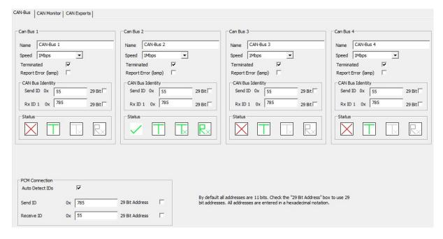
The CAN display screen shows status for each of the 4 available CAN bus:
