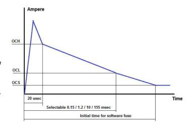
After the time interval INIT, the initial time from switching the output ON, the current draw must be below the user defined software fuse level, OCS. If the current draw exceeds this threshold, the output will be switched off.
