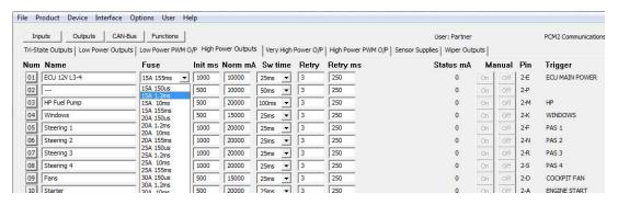
The driver stages can deliver significantly more current, but it is important to avoid overloading the wiring and contacts in the connector.
