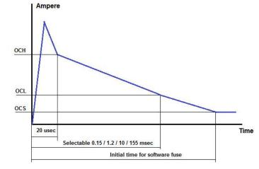
in "NORM mA". This interval must exceed the time interval selected for OCL, suggested value > 200 msec.
