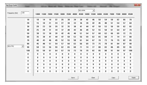
Use the drop down menus to select the channels used for the X and Y axis of the table. It is not necessary to use the full table and all breakpoints in the maps nor to use both axis's. Using a two-axis calibration, start filling the map out from upper left hand corner. Using a single axis calibration, select the X or Y-axis as the input reference, using only the first row or column of the other axis.
