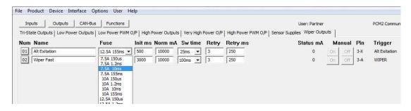
The driver stages can deliver significantly more current, but it is important to avoid overloading the wiring and contacts in the connector.
