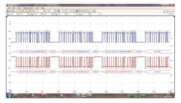
If the CAN bus is incorrectly terminated, having only one single termination resistor, the data transfer will be instable. Please note the shift in voltage level and wave forms:
