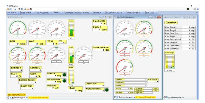
By selecting the various tabs, you can view and edit settings for fuel and spark, oil pressure control, variable camshaft timing, lambda fuel control, idle speed, monitor ignition coil currents and diagnose the drive-by-wire throttle body.
