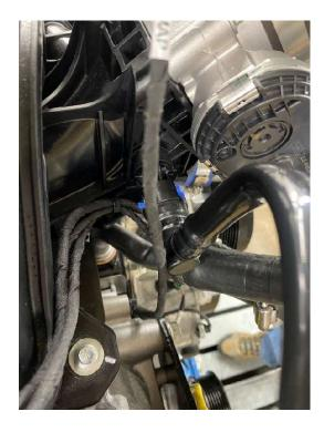
Secure the connections to CHT, VCT and the cam sensor on the front cover:
