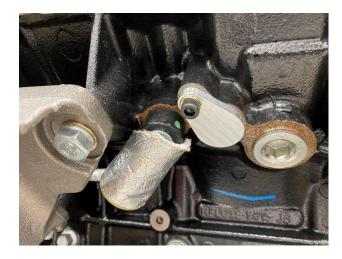
The two water pipes on the front of the engine is for the car heater. If you do not use these connections for the heater, one of the two heater pipes on the front of the block can easily be blocked off as well:
