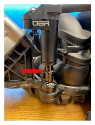
Carefully push the adaptor down onto the nipple, make sure the adapter slides all the way down over the nipple.
