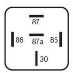
It is strongly recommended to let the ECU control your fuel pump relay. We updated the power harness in July 2022 to include a dedicated fuel pump relay. The kit includes a relay and two terminals for the fuel pump wires but not the wires. The wires must be minimum 16 gauge.
