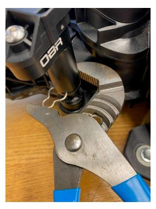
Insert the spring clip into the slot, make sure it grabs the intake manifold nipple below the lock ring and now press it into its lock, make sure it is fully inserted and that the adapter is kept safely in its place. Plug the 4-way connector with the orange seal into the sensor.
