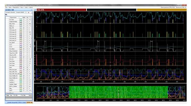
The Charting Tool is a graphic data analysis tool, displaying recorded data in a strip chart mode. It can display data from both the ECU's with on-board data recording as well as the ECT logger tool.
