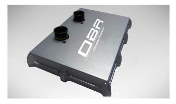
Communication with the EFR14 is carried out over one of two CAN Bus.
